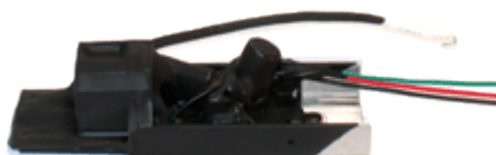
Figure 4-4: High Voltage Supply
