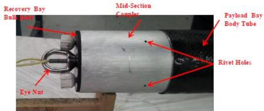
Figure 2: Mid-Section Coupler/ Recovery Bay Bulk Plate
