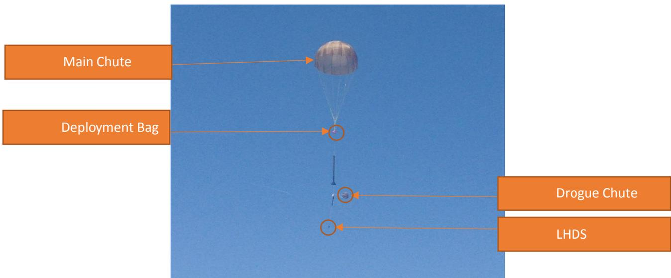
**Figure 2-3: Main Chute Deployed**
