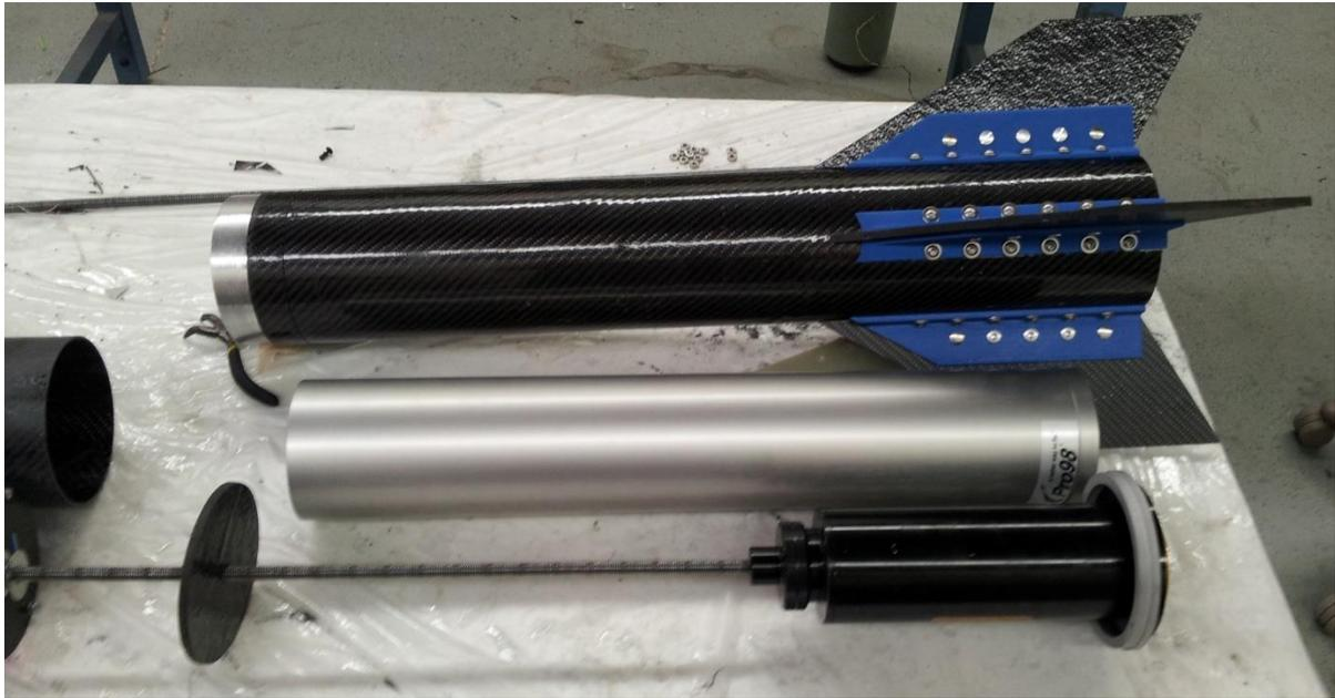
**Figure 1-7: Fin Can and Motor Cases**
