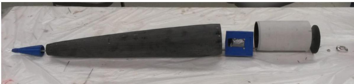
Figure 1-3: Nosecone Assembly
