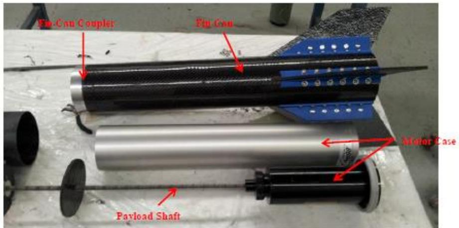
Figure 5: Fin Can Section
